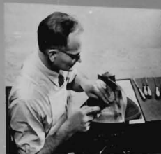
THE SHOP'S LATEST DEVELOPMENT IS THE CASTING OF METAL MASTERS FOR SUPERSONIC NOZZLES. WITH A LOW MELTING ALLOY, THIS METAL IS A TEN-BEIGHTH ALLOY AND CAN BE WORKED WITH WOODWORKING HAND AND MACHINE TOOLS.
