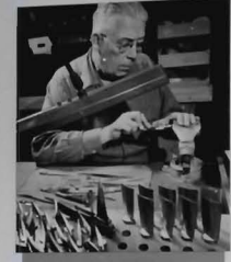
5. FINAL INSPECTION OF THE BLADE
