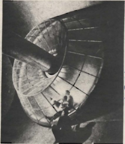
SCREENED INLET OF COMPRESSOR NO. 2
