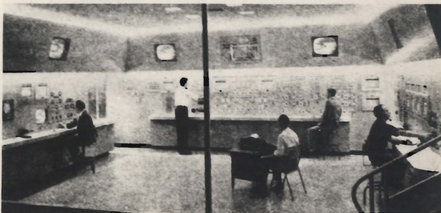
WIND TUNNEL CONTROL ROOM —The control room of the Lewis unitary plan wind tunnel. The tunnel diagram (top, center) provides a pictorial indication of the position of each of the major valves controlling tunnel operation. Each of the 24-inch television monitors (near ceiling) can be connected to any of the three TV cameras that survey the tunnel.
