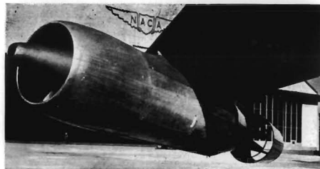
CORRUGATED nozzle in combination with annular sheet metal ejector is most promising noise suppressor being studied by the NACA. Ejector eliminates thrust loss due to the corrugated nozzle, but it has a large drag which would lower aircraft range.
