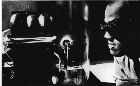
A small wheel is jet-operated by means of an ion-propulsion model.
