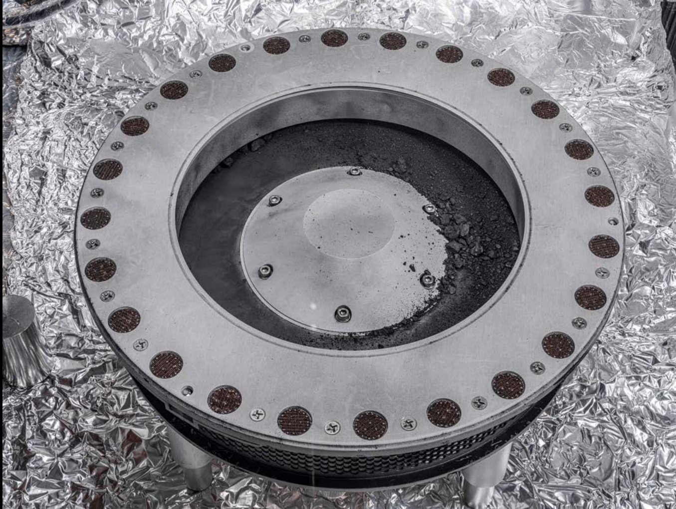
A view of the outside of the OSIRIS-REx sample collector. Sample material from asteroid Bennu can be seen on the middle right.
