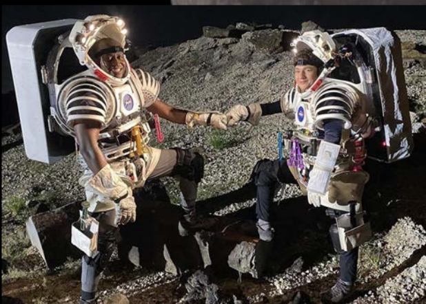
The Joint Extravehicular Activity and Human Surface Mobility Program Test Team (JETT) testing tools and spacesuits in a rock yard at NASA's Johnson Space Center, simulating the uneven terrain of the lunar surface, in preparation for Moonwalks
