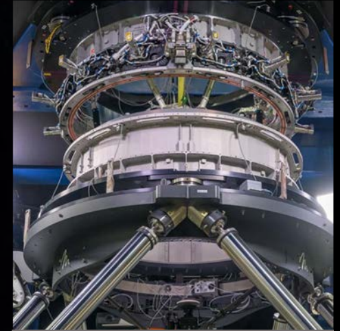
Starship Human Landing System docking system qualification test
