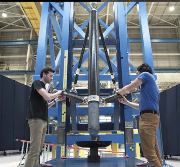
Blue Origin conducted a drop test of the Blue Moon MK1 cargo lander leg to provide engineers with data to correlate design models for dynamic loads analysis.
