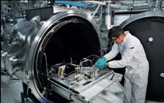
A Blue Origin technician conducts a vacuum chamber fit check for a fuel cell at Blue Origin's facility in West Texas.
