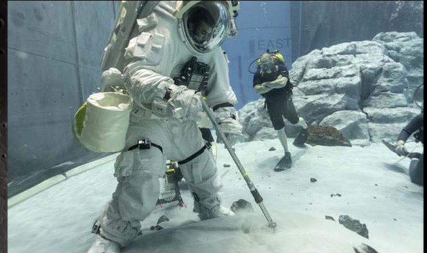
Spacesuit and hardware tests on the simulated lunar terrain on the Neutral Buoyancy Laboratory (NBL) pool floor
