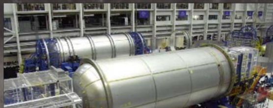
Hardware for Blue Origin's New Glenn second stage, which will refuel the cislunar transporter as part of Blue Origin's Artemis V architecture, is being manufactured at Blue Origin's production facility in Cape Canaveral, FL.
