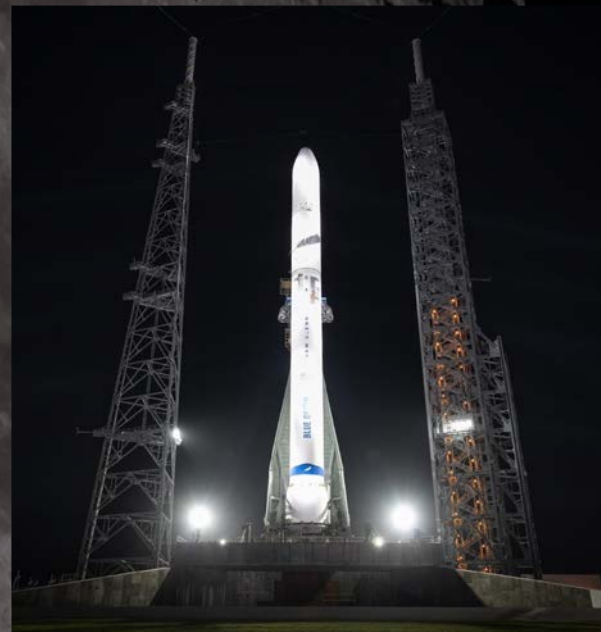
Blue Origin's New Glenn rocket upended on its launch pad for the first time. The rocket's first stage underwent three tanking tests in preparation for its first launch.
