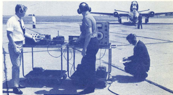
Measuring jet engine noise
