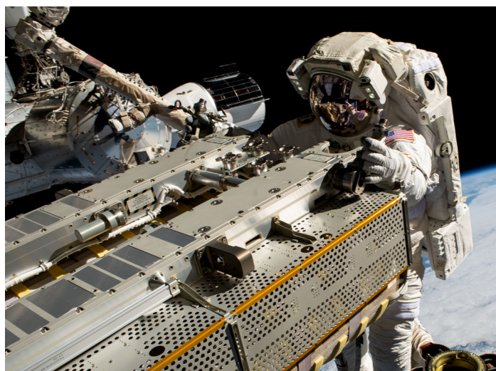
Figure 2. NASA astronaut and Expedition 68 Flight Engineer Woody Hoburg rides the Canadarm2 robotic arm while maneuvering a roll-out solar array toward the International Space Station’s truss structure for installation during a six-hour and three-minute spacewalk.
