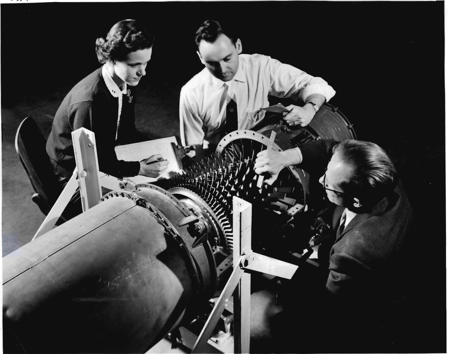
Special arrangement of the turbine with propeller to measure the torque of propeller on wind tunnel
