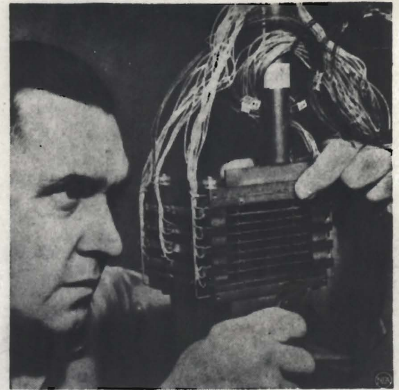
THIS MULTIPLE SANDWICH being adjusted by an NACA technician is a test unit to furnish data in designing heat exchangers which may some day be used in reactor for an atomic plane.
