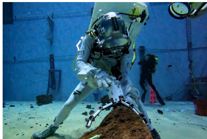
A NASA diver testing a student created tool in the Neutral Buoyancy Lab at Johnson Space Center as part of the 2022 Micro-G NExT challenge. Credit: NASA
