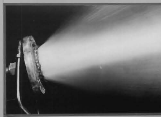
NEW DESIGN INJECTOR TYPES ARE TESTED IN TERMS OF BURNING PERFORMANCE FOR A VARIETY OF PROPELLANT TYPES.
