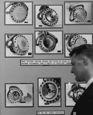
NEW DESIGN INJECTOR TYPES ARE TESTED IN TERMS OF BURNING PERFORMANCE FOR A VARIETY OF PROPELLANT TYPES.
