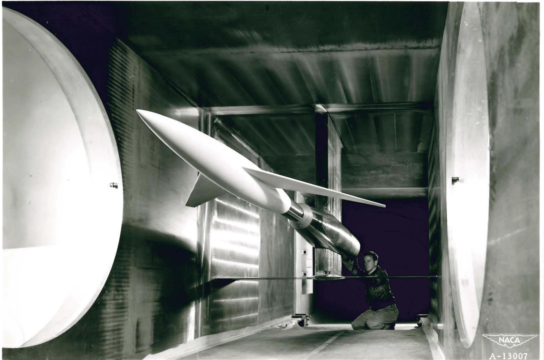
Model mounted in the test section of the 6- by 6-foot supersonic wind tunnel.
