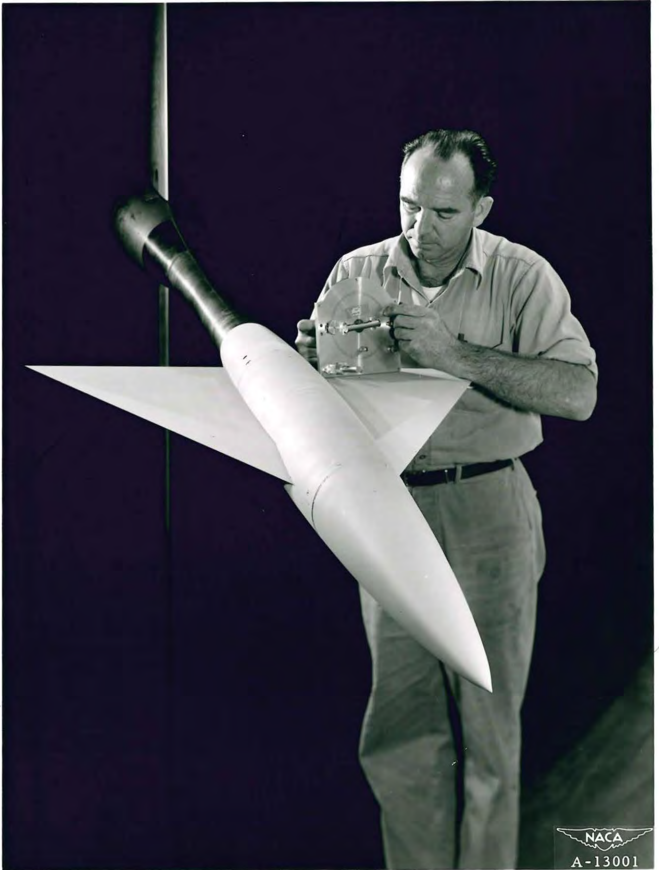
A triangular wing model mounted in the test section of the Ames 12-foot high-pressure wind tunnel.
