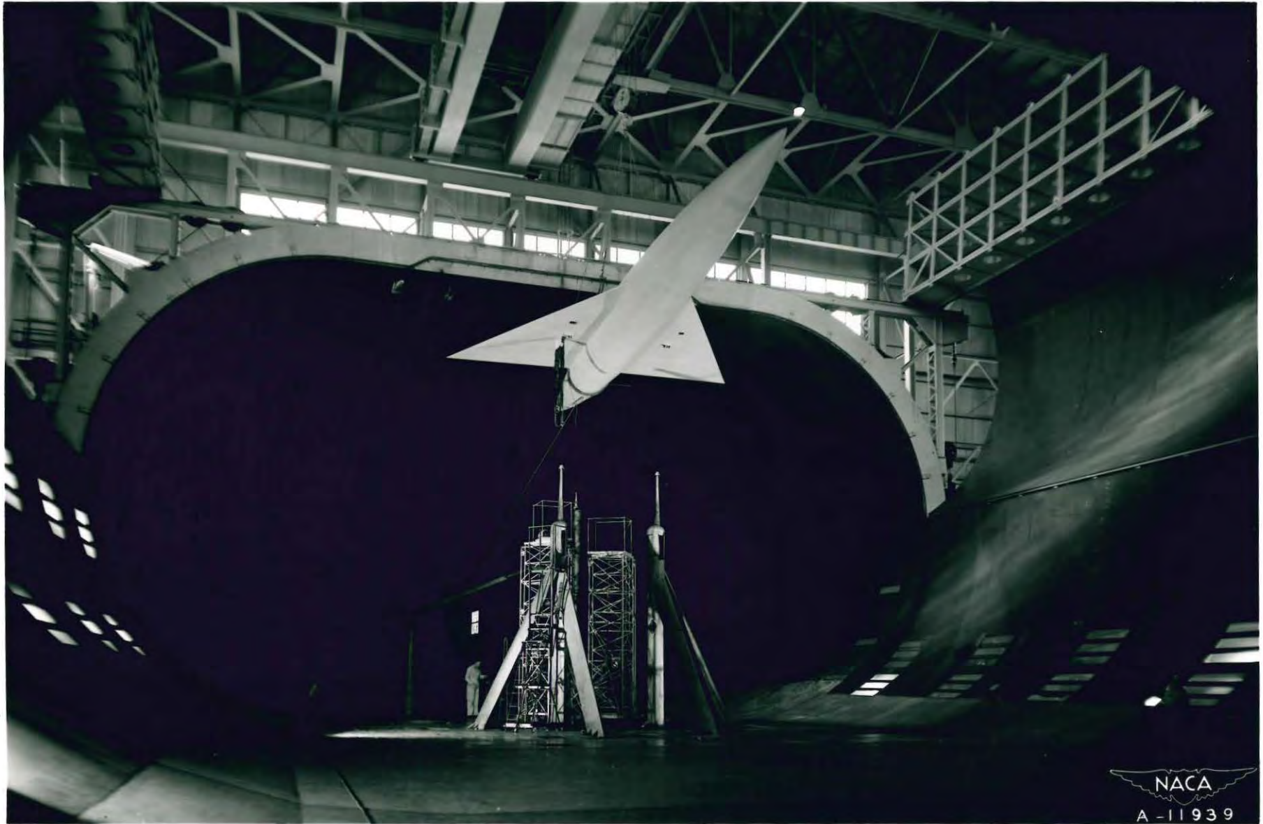
A triangular wing model being mounted in the Ames 40- by 80-foot wind tunnel.
