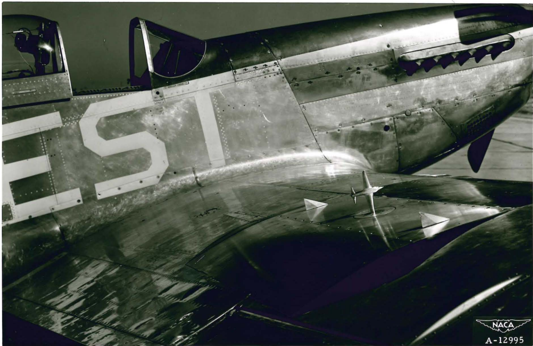
A close-up of the P-80 model mounted for testing at transonic speeds by the wing-flow method.
