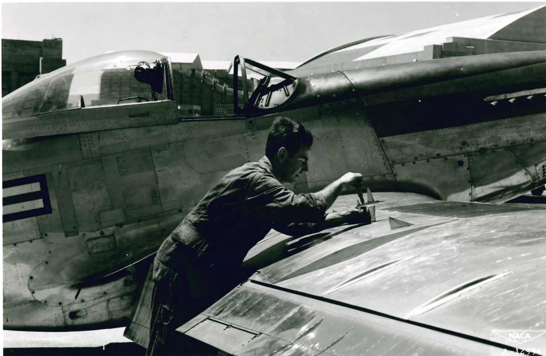
A model of the P-80 airplane being mounted on the wing of a P-51 airplane for wing-flow tests.
