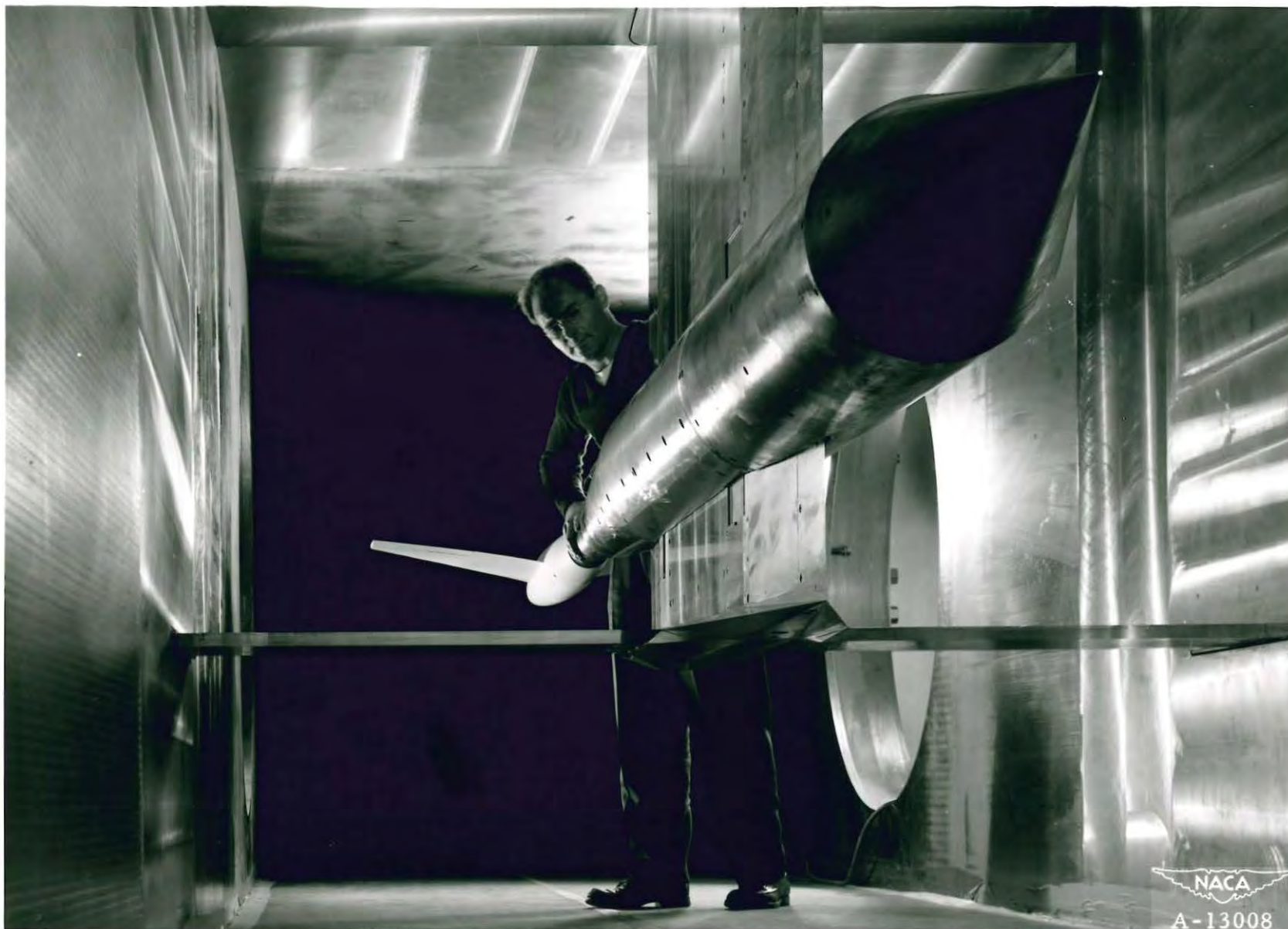
Rear-view of the model support in the 6- by 6-foot supersonic wind tunnel.
