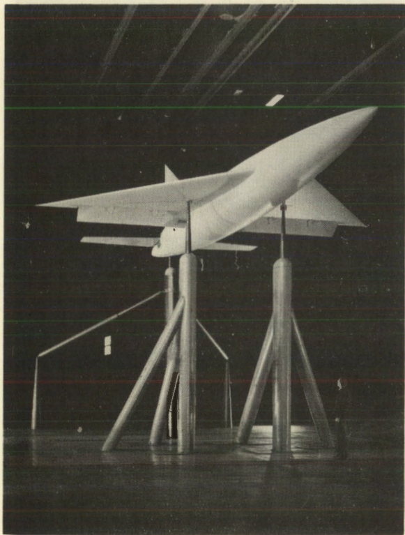
High-lift flaps studied in tunnel at full-scale.
