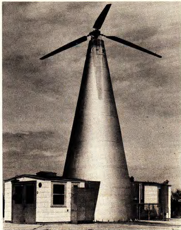
HELICOPTER ROTORS ARE INVESTIGATED FOR VERTICAL FLIGHT AND HOVERING PERFORMANCE ON THIS TEST TOWER AT THE LANGLEY LABORATORY. OTHER CHARACTERISTICS ARE STUDIED IN WIND TUNNELS AND IN FLIGHT.
