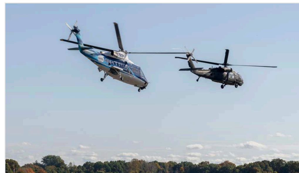
NASA and Sikorsky conducted flight tests from Sikorsky Memorial Airport in Bridgeport, Connecticut, to evaluate autonomous flight software systems designed for Advanced Air Mobility concepts. NASA/Steve Freeman
