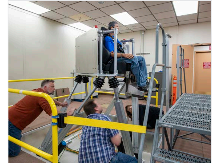
Researchers tested NASA Armstrong's newly installed motion simulator in April 2023. The simulator includes virtual reality goggles depicting an aircraft cabin and city environment, as well as noise and seat motion, to simulate an air taxi ride . NASA/Genaro Vavuris
