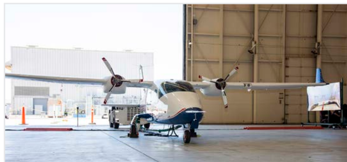
NASA's X-57 Maxwell all-electric aircraft project , which concluded aircraft operational activities in 2023, provides aviation researchers with hundreds of lessons learned, as well as revolutionary development in areas ranging from battery technology to cruise motor control design. NASA
