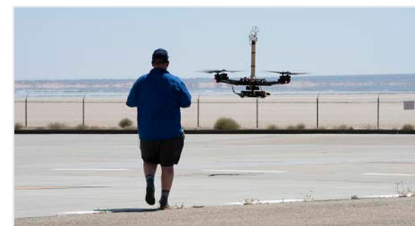
NASA Armstrong's Model Laboratory supported a campaign to measure wind at low altitudes to gather data needed to enhance air taxi safety. NASA/Carla Thomas
