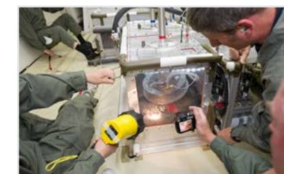
Evaluating OSIRIS-REx sampling system in microgravity via Flight Opportunities. NASA/James Blair
