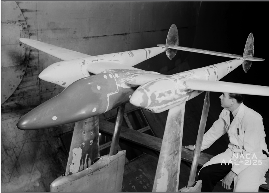
Figure 6: A test model variant of the P-38 showing its unconventional twin-boom configuration. (Image credit: NACA AAL-2125)
