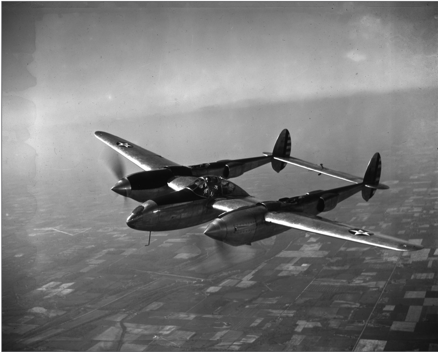
Figure 1: An early prototype of the Lockheed P-38 Lightning. The aircraft's performance moved into realms not seen before. Pilots experienced the forces of the transonic region on the aircraft and its control surfaces. (Image credit: NASM HGC-968)
