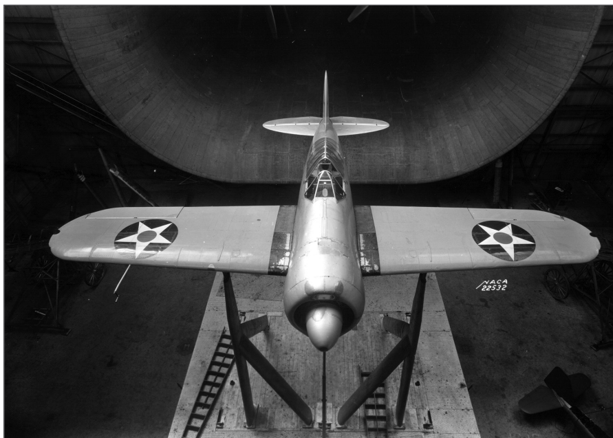
Figure 2: The Navy's Brewster Buffalo fighter was the first military aircraft to benefit from Langley's drag reduction program. This practical engineering research at Langley proved to be so successful that almost all American combat aircraft went through the full-scale tunnels to discover or improve their aerodynamic flaws. (Image credit: NACA 22532)
