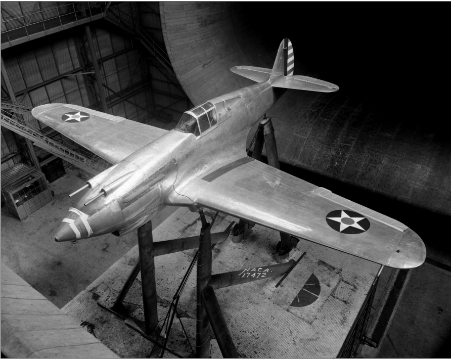
Figure 1: A Curtiss-Wright XP-40 prototype in the NACA Full-Scale Tunnel at Langley Field, Virginia, in April 1939. NACA engineers made a number of improvements to reduce the aircraft's drag characteristics; these included combining the radiator and oil-cooling air scoops, as well as changes to the exhaust manifolds and landing gear doors. These small changes resulted in an increased air speed of 53 miles per hour. (Image credit: NACA 17472)
