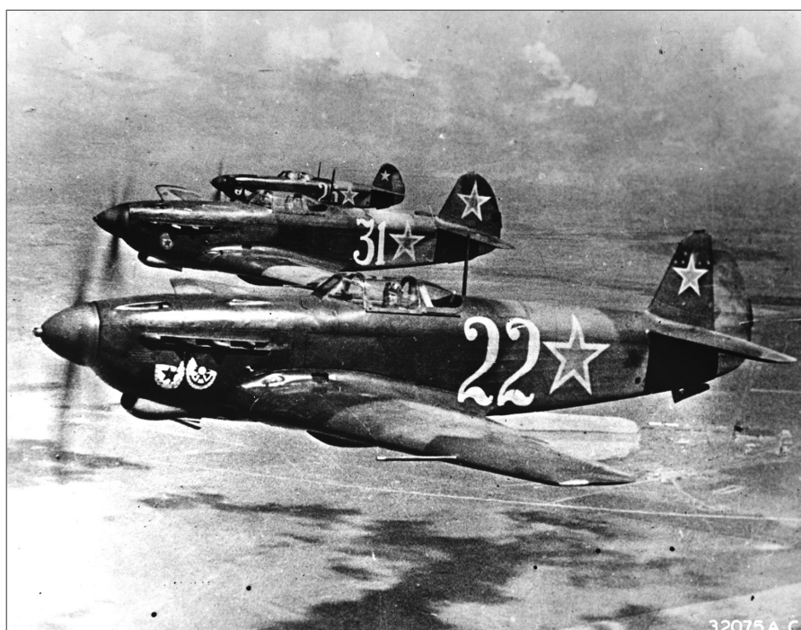
Figure 2: TsAGI's recommendations to clean up the aerodynamics of the Yak-7B resulted in the excellent Yak-9 fighter. The long-range Yak-9D, shown here, featured mixed wood and metal construction and was a match for contemporary Messerschmitt Bf 109s and Focke Wulf Fw 190s. (Image credit: National Air and Space Museum, Smithsonian Institution, image NASM 85-17696)
