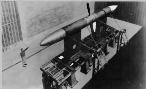
PROPELLER DYNAMOMETER ON GROUND TEST STAND
