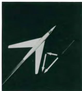
(c) Velocity components on swept-back wing.
