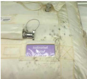
Fungal contamination of the fabric of a Contingency Water Container bag
