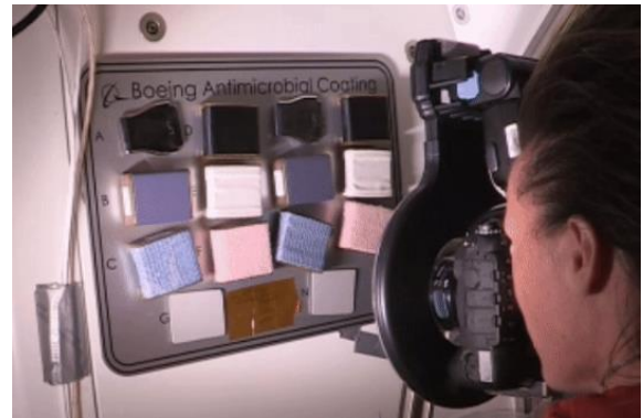
Touch panels installed for the ISS Boeing Antimicrobial Coating investigation. Space Station 101: Microbiology , NASA
