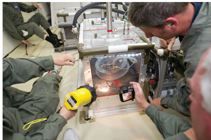
Evaluating OSIRIS-REx sampling system in microgravity via Flight Opportunities. Credits: NASA/James Blair
