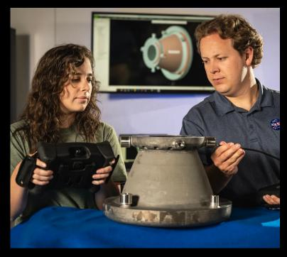
Additively Manufactured Rocket Engine Nozzles
