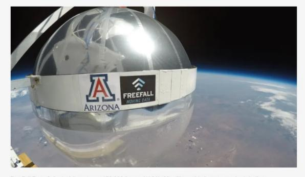
FreeFall Tests Spherical Antennas at 159,000 feet on NASA's 60 million cubic foot stratospheric balloon. Dr. Christopher Walker, NIAC Fellow / FreeFall Aerospace
