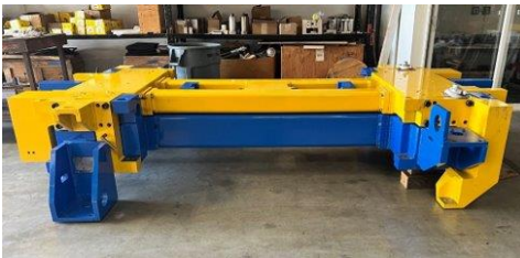
PSL Thrust Stand Refurbishment
