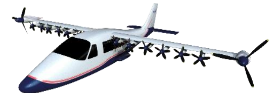
Flight test with integrated DEP motors and folding props (cruise motors remain on wing-tips)
