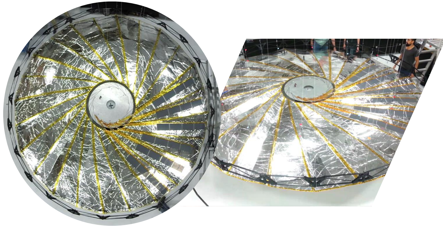
Deployed 5m flight-like optical shield inside truss
