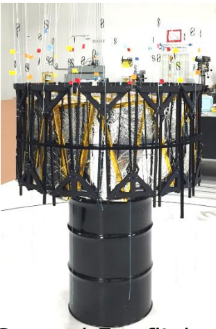
Stowed 5m flight-like optical shield inside truss
