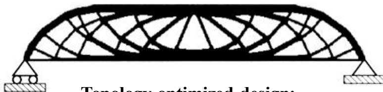
Topology optimized design: ~ 42% stiffer for same weight
