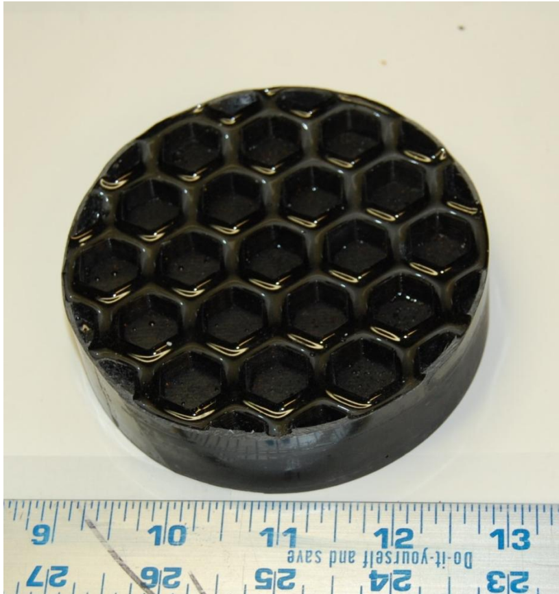
Molded back structure using molds from the Virginia Tech DREAM Lab
