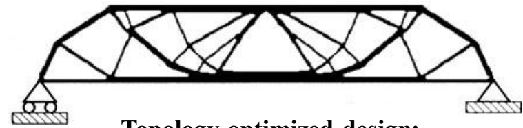
Topology optimized design: ~ 48% lighter for same (elastic) stiffness
