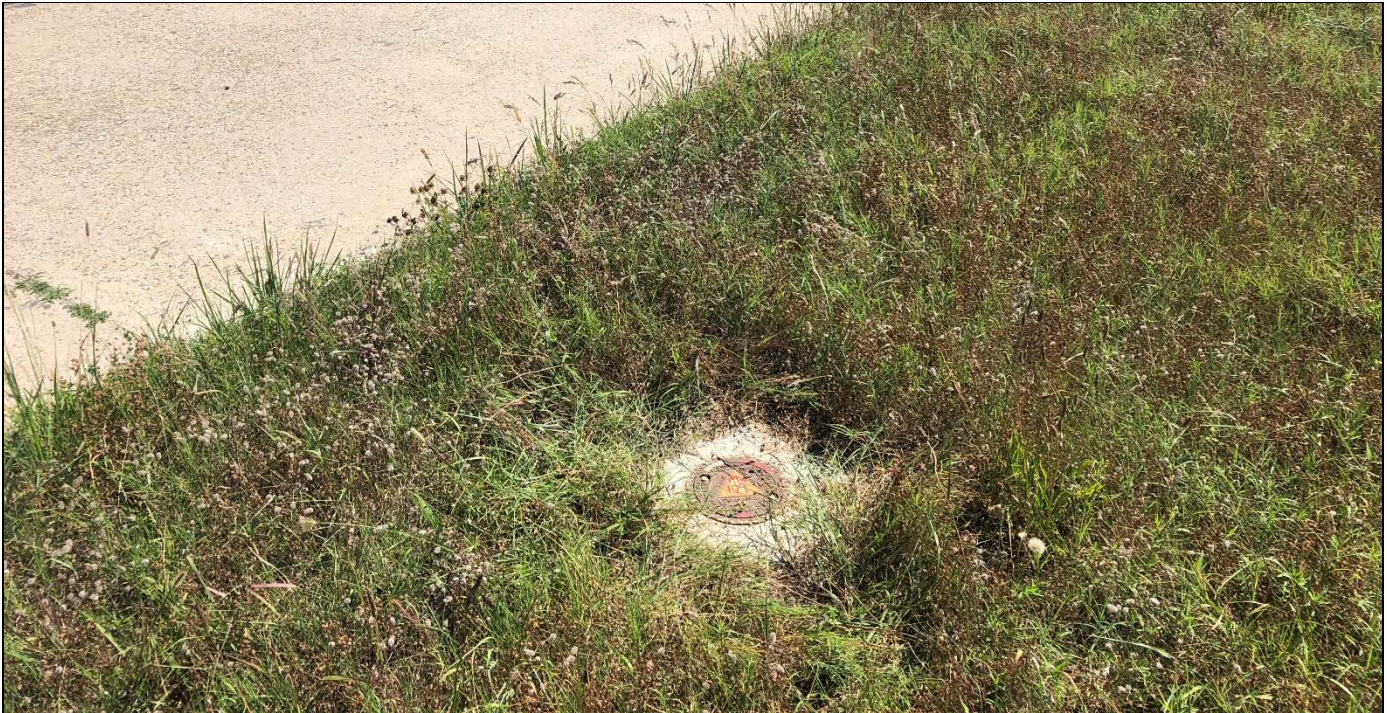
View of FFTA-MW109. Flush mount completion in grass on south side of abandoned taxiway.
