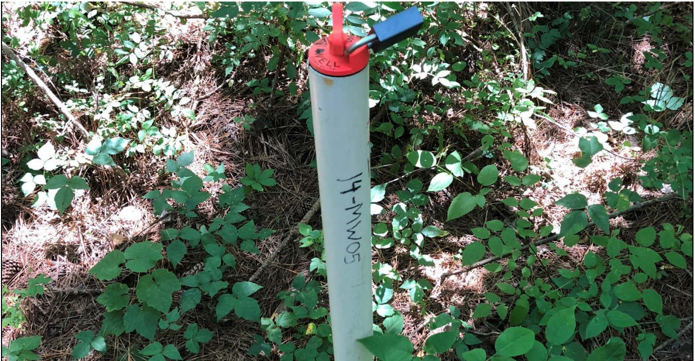
View of 14-MW005. There is no protective casing installed for this well due to the location.
