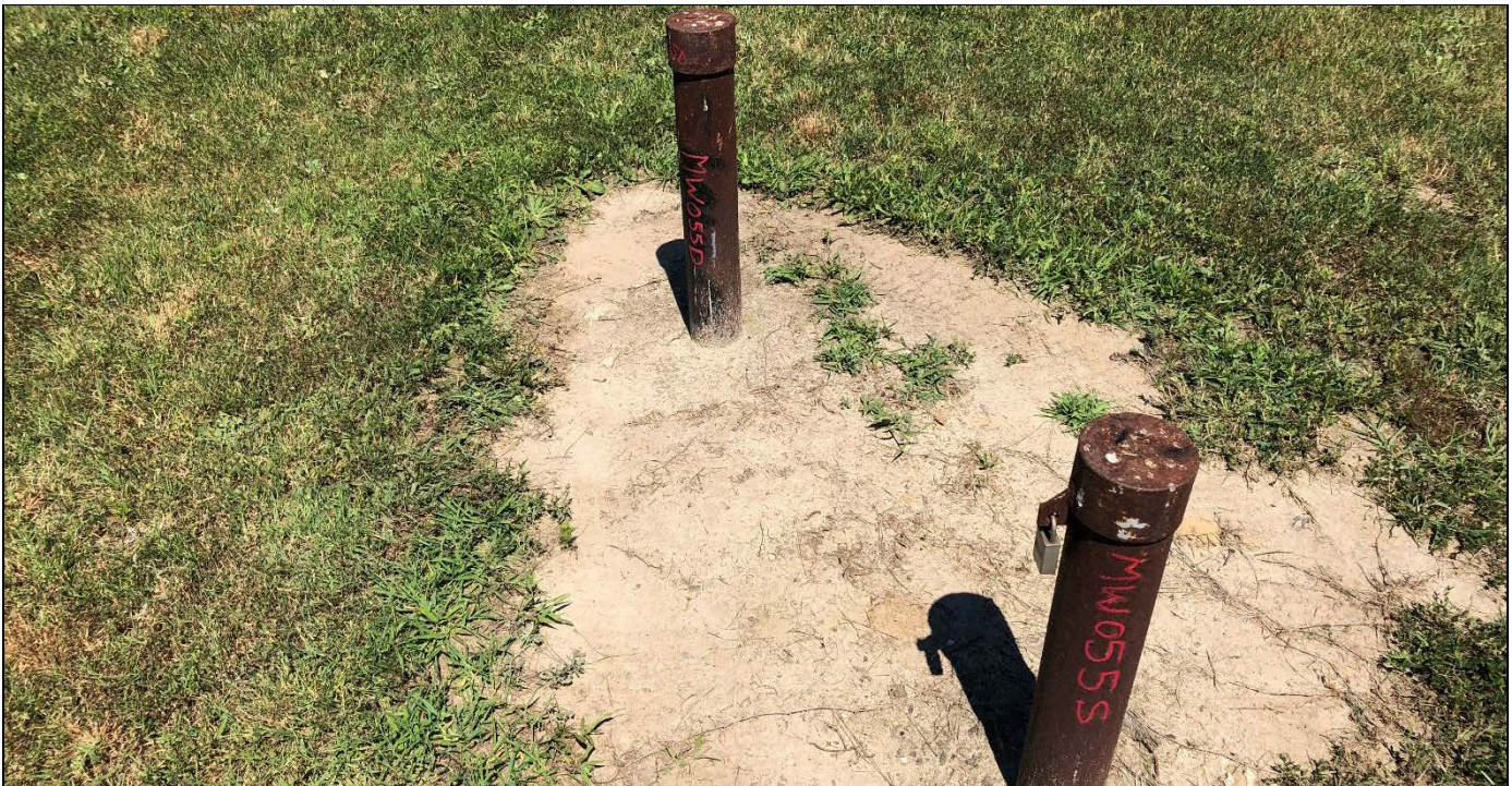
View of FFTA-MW055S and FFTA-MW055D. Other than some rust the well are in good condition.
