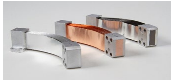
Figure 7.4: Thermal strap design with aluminum foils, copper foils, and PGS in aluminum end blocks (above), and their respective measured thermal conductance (left). The dashed lines connecting data points are based on material thermal conductivity curves. Credit: SDL.
