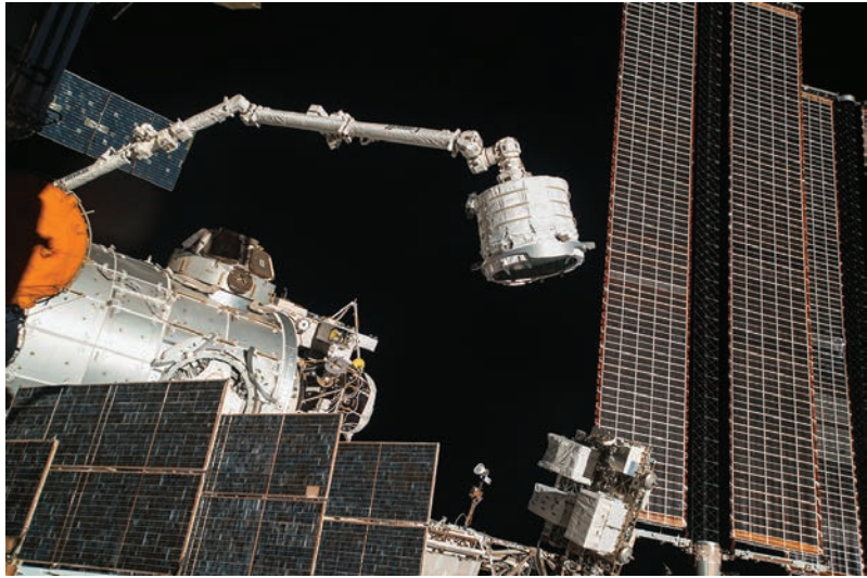
Figure 8. BEAM being installed on the ISS by the Canadarm
