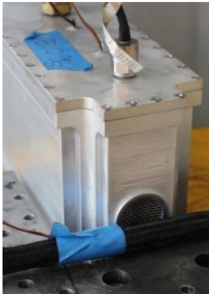
Batteries instrumented with Pressure Transducer and Thermocouple
