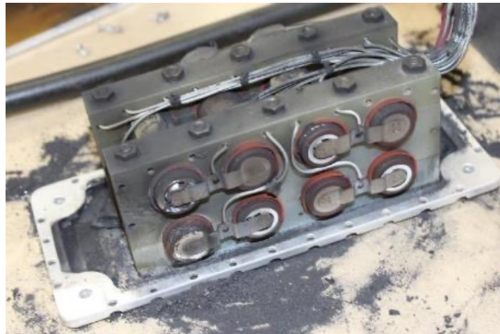
Cell tab interconnects remained in contact for all cells including the vented cell No propagation was observed
