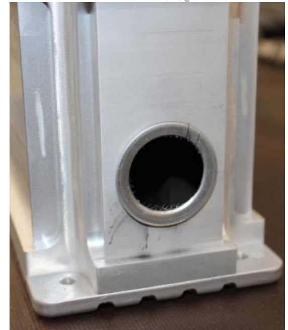
Oxidization of Aluminum screen after cell vent process
