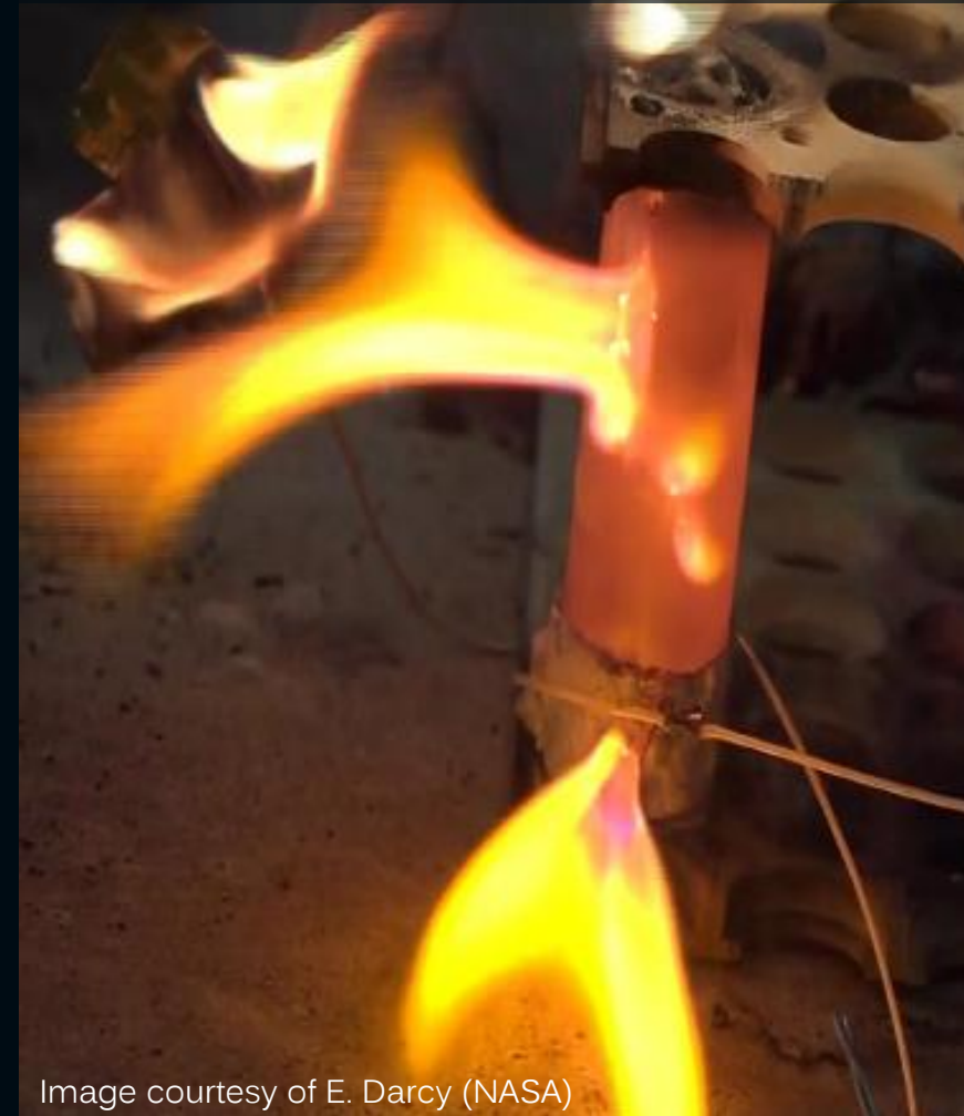
Hazardous flare stemming from breach
