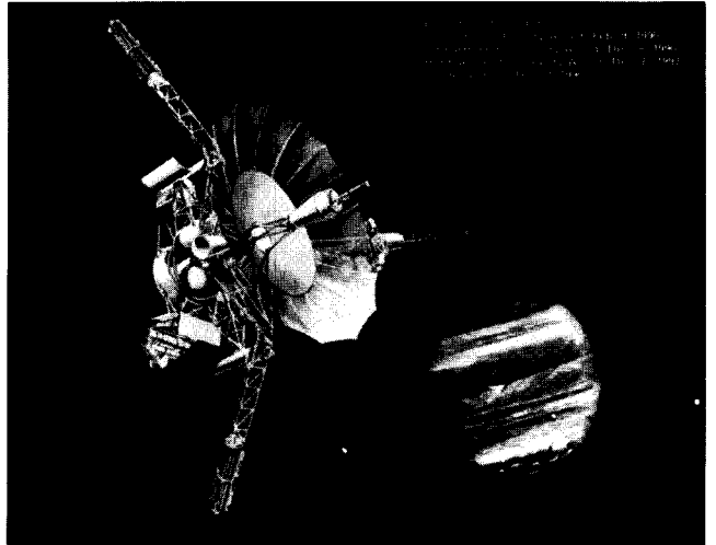
Artist's concept of Galileo spacecraft to Jupiter using General Purpose Heat Source Radioisotope Thermoelectric Generators.
