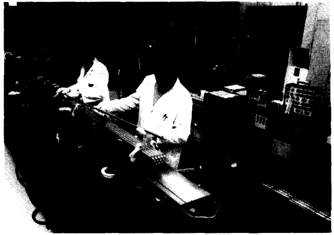
Preparation for testing SP-100 fuel pins in the Fast Flux Test Facility at Hanford, WA, for the Los Alamos National Laboratory.
