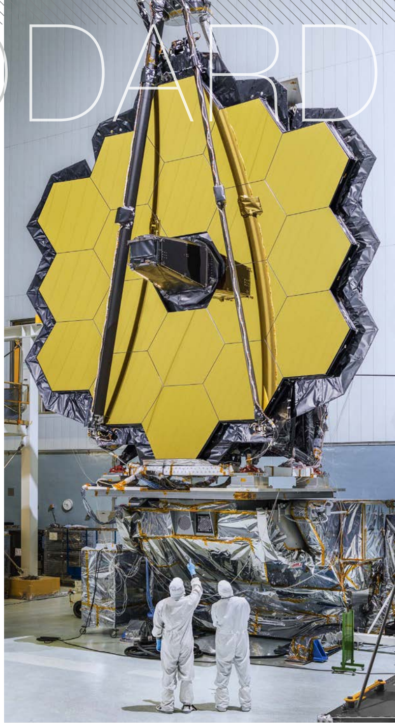
The primary mirror of NASA's James Webb Space Telescope consisting of 18 hexagonal mirrors looks like a giant puzzle piece standing in the massive clean room of NASA's Goddard Space Flight Center in Greenbelt, Maryland. (NASA/Goddard/Chris Gunn)
