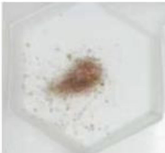
Li Metal Soaked in Fluoromethane
