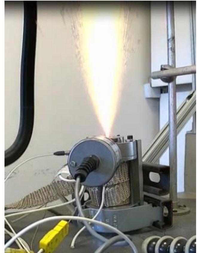
Demonstration of proof of concept. A COTS Li-ion cell used in the Aerocube satellites was heated to thermal runaway, and the gasses were focused through a nozzle to generate thrust.
