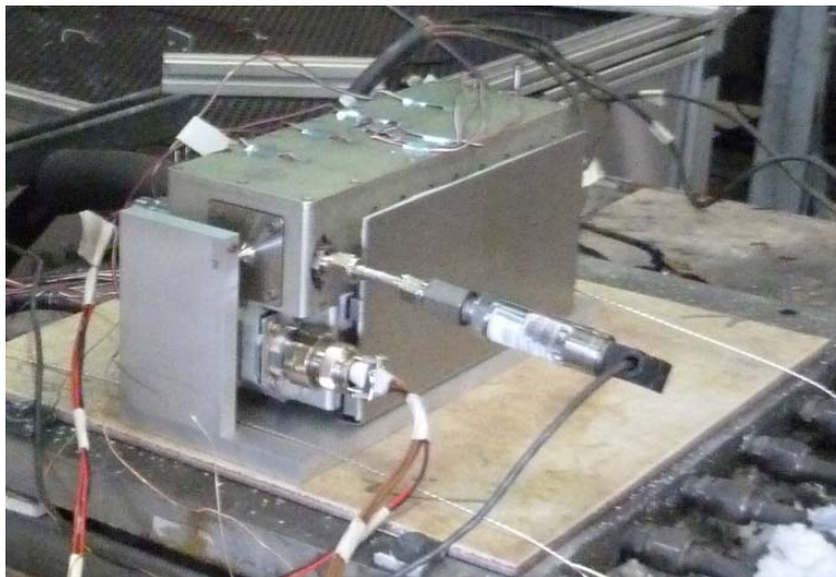
Test Article with Fabric Suspended in front of Housing Vent Ports
