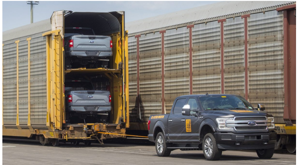
2019, Ford F-150 Fully electric truck with a lithium-ion battery ; Power: tows 1.25 million lb. train
