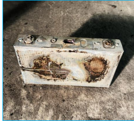
25 Ah Li-ion NMC prismatic cell, 95 Wh
