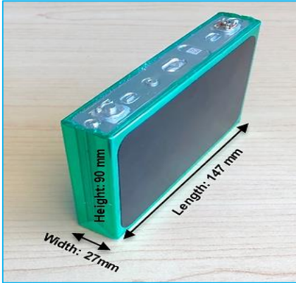
25 Ah Li-ion NMC prismatic cell, 95 Wh
