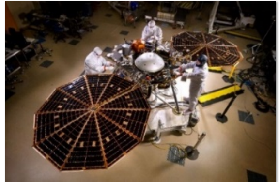
Figure 26. Technicians work on NASA's InSight lander during a solar array deployment test. The lander will use solar power to operate its science equipment on the surface of Mars. (NASA)
