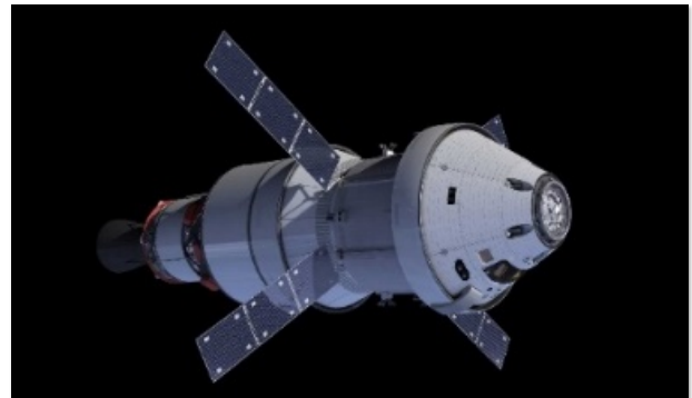
Figure 1. Illustration of the Orion Spacecraft, a multi-purpose crew vehicle designed to carry astronauts into deep space. (NASA)
