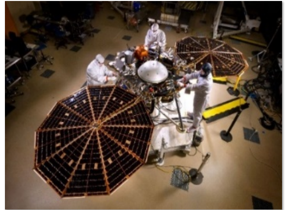
Figure 6. Technicians work on NASA's InSight lander during a solar array deployment test. The lander will use solar power to operate its science equipment on the surface of Mars. (NASA/JPL-Caltech/Lockheed Martin)
