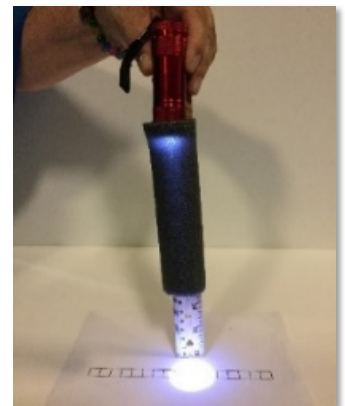
Figure 20. Conducting the investigation. The ruler is behind the flashlight in the foam insulation.
