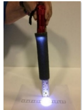
Figure 29. Conducting the investigation. Ruler is behind flashlight and foam pipe insulation tube.
