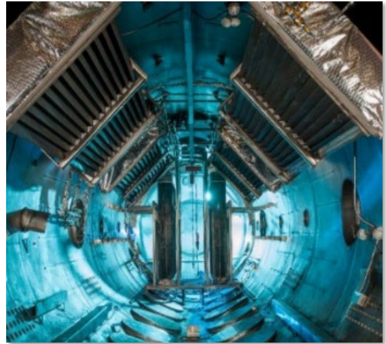
Figure 18. Vacuum Chamber 5 (VF-5) at NASA's Glenn Research Center provides an environment that simulates space-like conditions. VF-5 has been used to test electric propulsion systems and power systems for in situ resource utilization.
