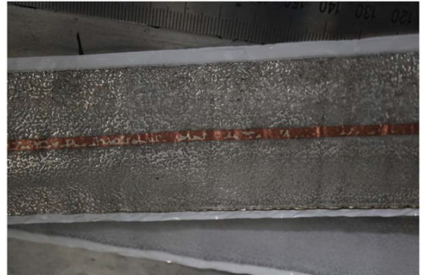
Discharged at 250 mA and 20°C (~19 Ah)
