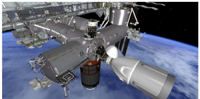
SpaceX Dragon docked to PMA. Crew translates through Dragon overhead hatch and PMA APAS hatch into ISS.
