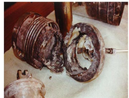
Remains of the solid fuel oxygen generator that combusted aboard Mir space station in 1997.
