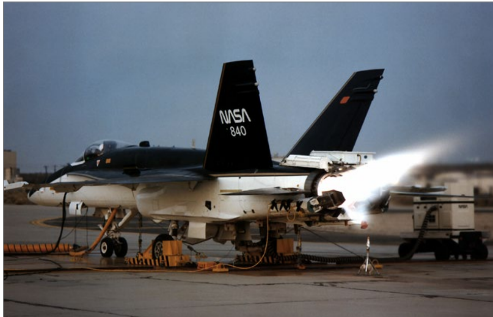
↑ The F/A-18 HARV is tied down for a thrust-vectoring demonstration using the afterburner to illustrate the engine's redirected exhaust. (Photo credit: NASA)
