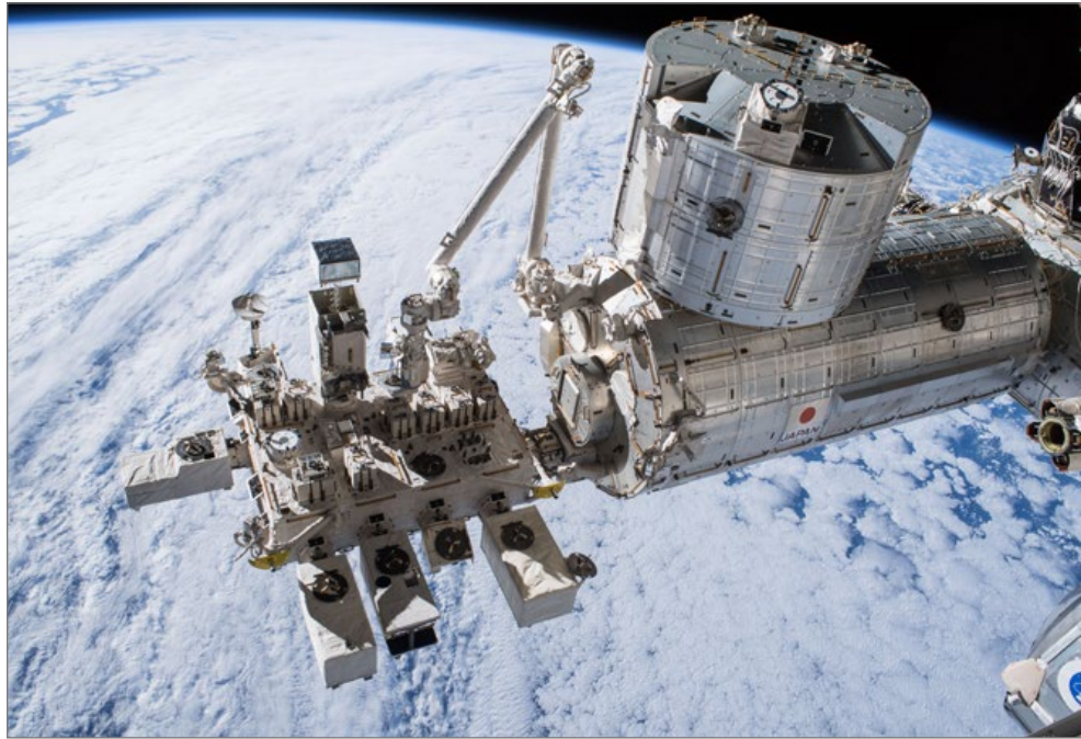
↑ JAXA's Kibo laboratory module (composed of a pressurized module and exposed facility, a logistics module, a remote manipulator system, and an inter-orbit communication system unit) is pictured in 2018. (Photo credit: NASA)
