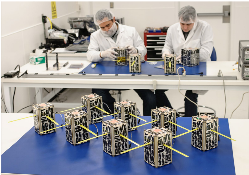
Completed EDSN Flight Units with Engineers Inspecting EDSN Flight Spares
