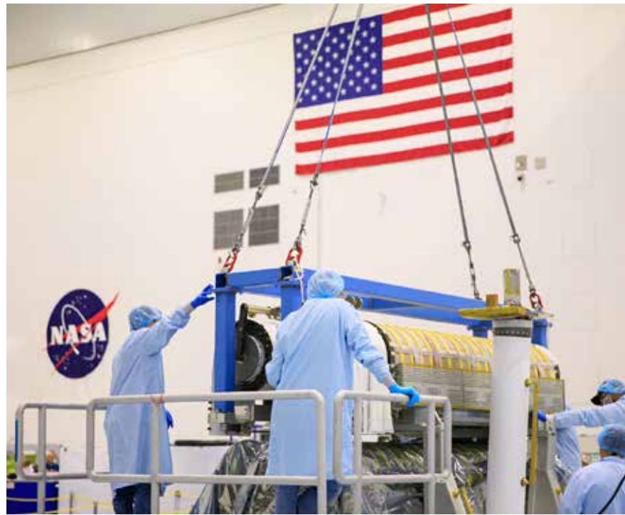
Inside the Space Station Processing Facility high bay at NASA's Kennedy Space Center in Florida, technicians assist as a crane lowers a set of International Space Station Roll Out Solar Arrays (iROSA) onto a platform on March 23, 2023. Photo credit: NASA/Isaac Watson
