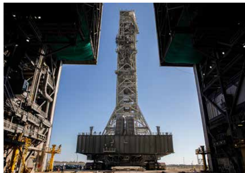
A view from inside the Vehicle Assembly Building at NASA's Kennedy Space Center in Florida on Dec. 9, 2022, as the mobile launcher, carried atop the crawler-transporter 2, arrives at the entrance to the transfer aisle, following the successful launch of the agency's Space Launch System (SLS) rocket and Orion spacecraft on the Artemis I flight test on Nov. 16, 2022. Photo credit: NASA/Ben Smegelsky
