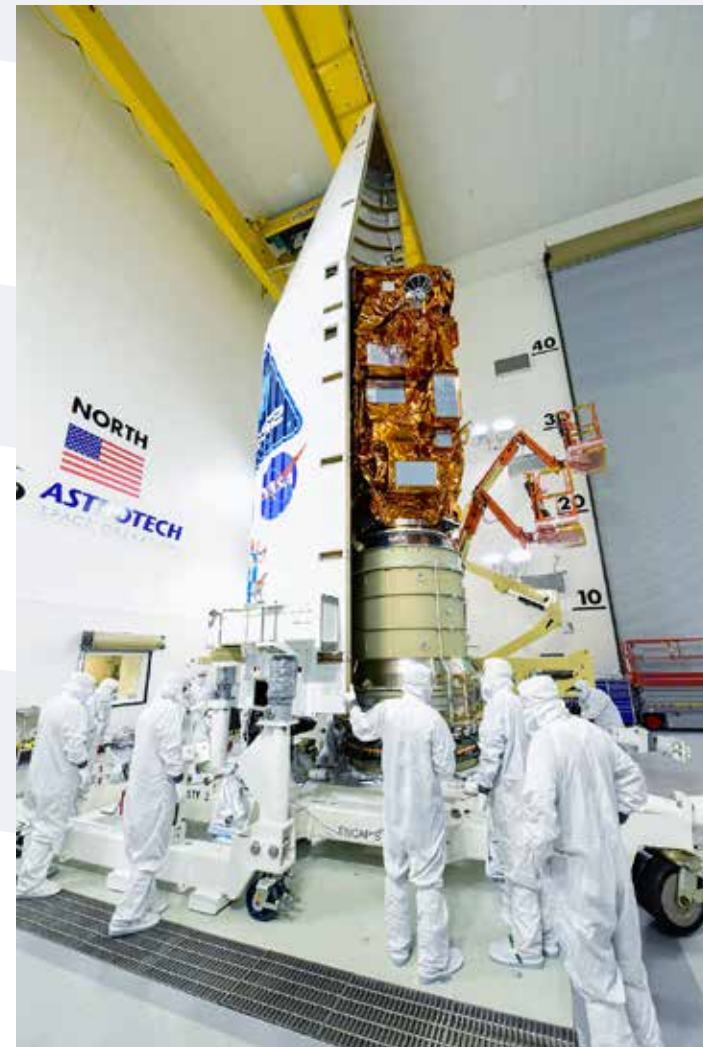
Technicians move the National Oceanic and Atmospheric Administration's Joint Polar Satellite System-2, stacked atop NASA's Low-Earth Orbit Flight Test of an Inflatable Decelerator secondary payload, into the first half of the United Launch Alliance Atlas V payload fairing inside the Astrotech Space Operations facility at Vandenberg Space Force Base in California on Oct. 12, 2022. Photo credit: USSF 30th Space Wing/Steve L. Ge
