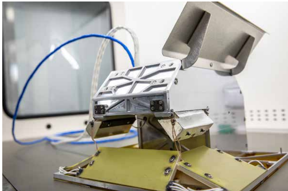
Inside of the Electrostatics and Surface Physics Laboratory, an electrodynamic dust shield (EDS) is in view on Jan. 18, 2023. The dust shield is one of the payloads that will fly aboard Firefly Aerospace's Blue Ghost lunar lander as part of NASA's Commercial Lunar Payload Services (CLPS) initiative. Photo credit: NASA/Cory Huston
