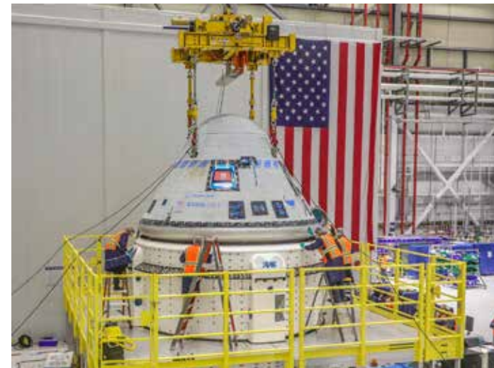
The Starliner team works to finalize the mate of the crew module and new service module for NASA's Boeing Crew Flight Test. Photo credit: Boeing/John Grant
