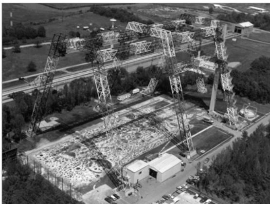
Lunar Landing Research Facility with simulated Moon surface used for astronaut training. (NASA photo)
