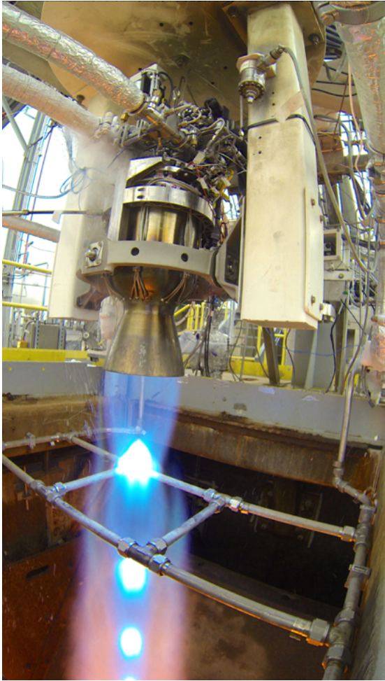
NASA engineers conduct a test of Project Morpheus's HD4B-LT engine at the E-3 Test Stand at Stennis Space Center on 20–21 February 2014. (NASA photo)
