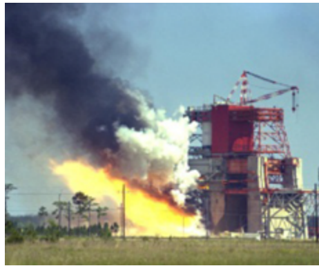
The first stage of a Saturn V rocket undergoes a hot-firing on the B-2 stand in 1967 at the then-MTF.
