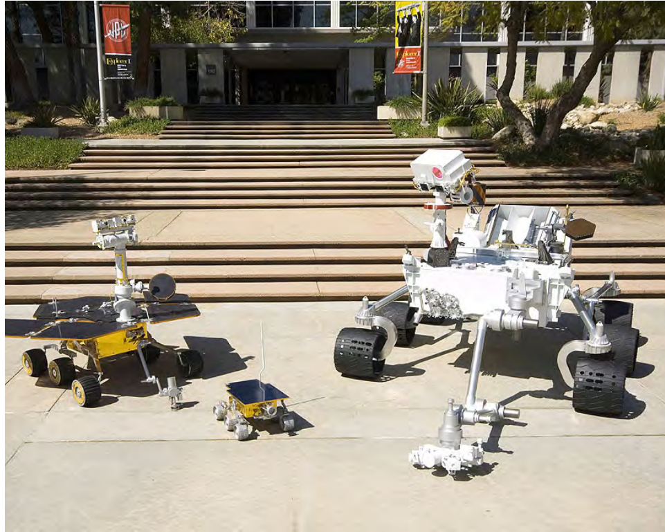
The Mars rovers in a family photo: Mars Science Laboratory's Curiosity rover (right), Mars Exploration Rovers (MERs) Spirit and Opportunity (left, only one pictured), and Mars Pathfinder's Sojourner (center). The rovers have increased in size to carry more scientific instrumentation and travel longer distances. (NASA/JPL-Caltech)
