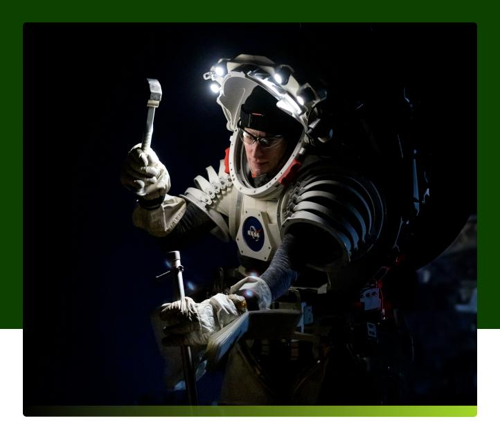
NASA astronaut Kate Rubins uses a hammer to get a drive tube into the ground to collect a pristine soil sample during a nighttime simulated moonwalk in the San Francisco Volcanic Field in Northern Arizona on May 16, 2024. The drive tube is the key piece of hardware for preserving the integrity of samples from the Moon.
