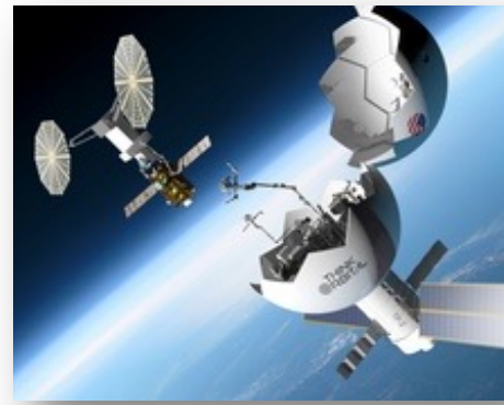
ThinkOrbital – A system to robotically assemble and weld very large pressurizable modules for CLDs in-space
