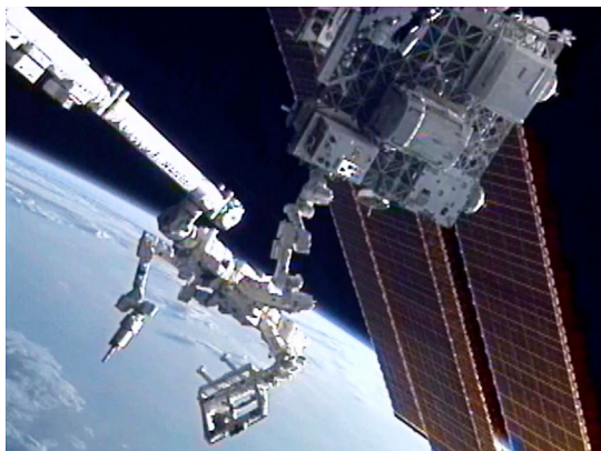
Dextre (center) practices a servicing task on RRM (above).
