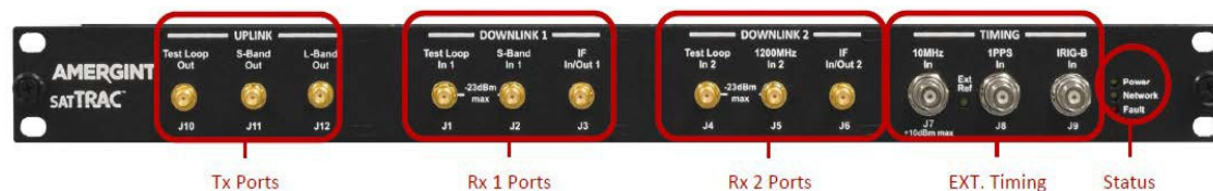
satTRAC Signal Converter Front View (1200 MHz Gen 2)
